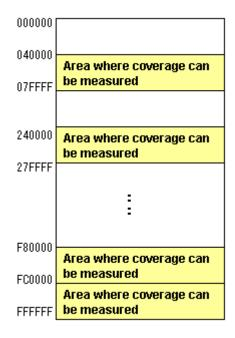
Figure 5.74 Schematic of coverage memory allocation
